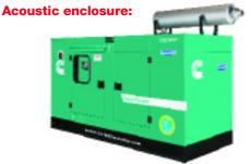
The acoustic enclosure is made of 1.6 mm thick CRCA sheets in Munsel green shade and a structural/ sheet metal base frame painted in black. The walls of the enclosure are insulated with fire retardant foam so as to comply with the 75 dBA at 1 mtr sound levels specified by Ministry of Environment & Forest.
